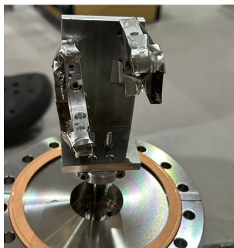
Figure 2. Newly installed EUV multilayer mirror monochromators.
