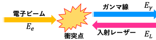
Figure 1. Schematic diagram of Laser Compton Scattering
