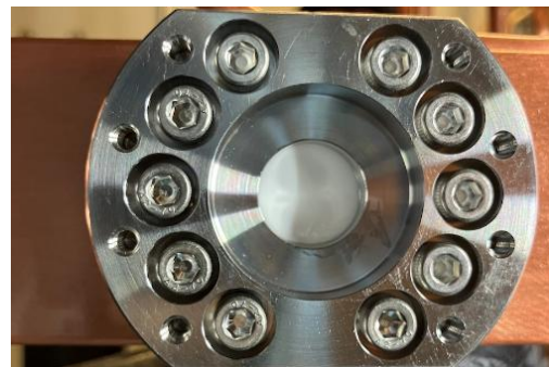
Figure 3. Ceramic section of the RF detector connected to the CB2 dummy load.
