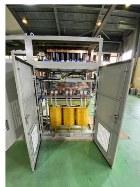
Figure 8. The new power supply for the bending magnets of the storage ring, manufactured by NICHICON CORPORATION.
