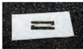
Fig.3 Integrated PTFE pattern obtained by the SR direct etching process. Two 3-dB couplers are cascaded.
