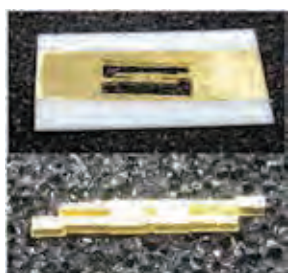
Fig.4 Integrated PTFE pattern covered with Au film by the sputter deposition and electroplating.
