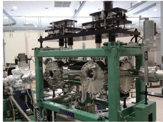
Fig. 5. Picture of two-focusing-mirror system of BL-07B.
