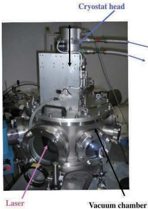
Fig. 4. Illustration and photograph of the translating cryogenic target system.
