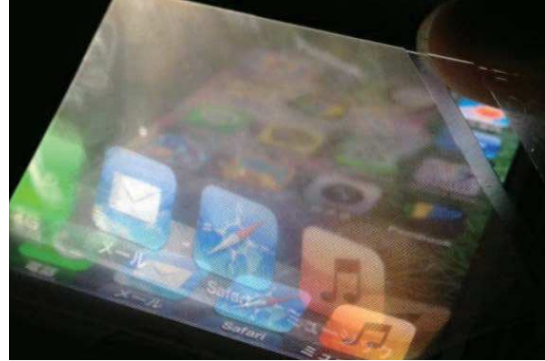
Figure 4. Floating image formed by the DCRA fabricated by X-ray lithography process using synchrotron radiation facility BL-2 at NEWSUBARU.
