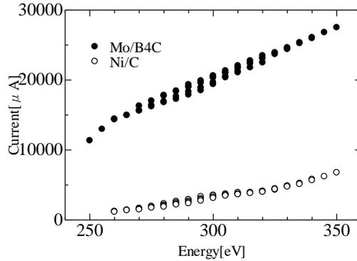
Fig. 5 PD current at 7th harmonic light with a Ag filter.
