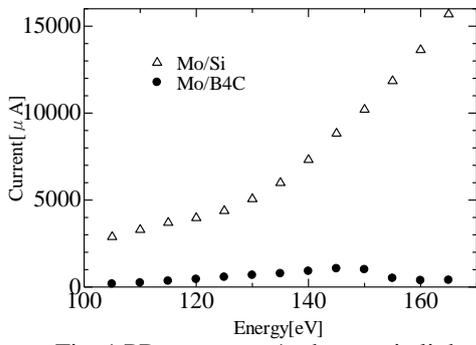
Fig. 1 PD current at 1st harmonic light without filter.
