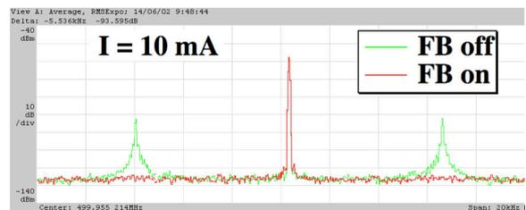
Figure 1: Measured time spectrum of the beam structure with and without feedback of synchrotron oscillation. The center line was the rf frequency and the broad side bands were synchrotron oscillation.
