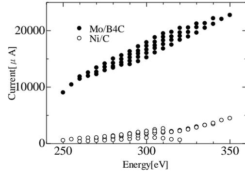
Fig. 4 PD current at 5th harmonic light with a Ag filter.
