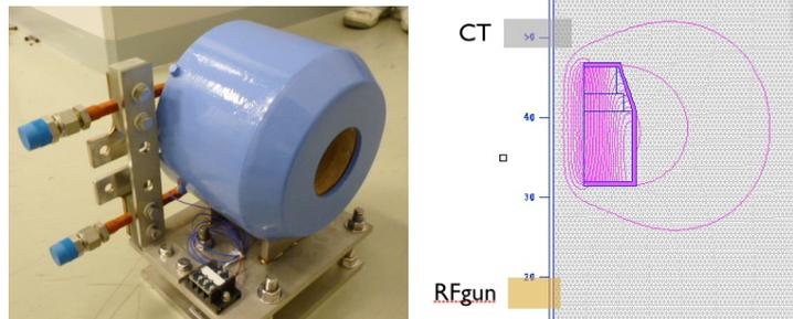
Fig.2 Solenoid coil (left) and 2D axial symmetric magnetic field calculated using POISSON code (right).
