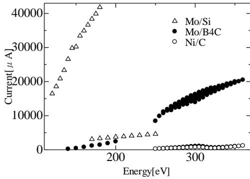
Fig. 3 PD current at 3rd harmonic light with a Ag filter.
