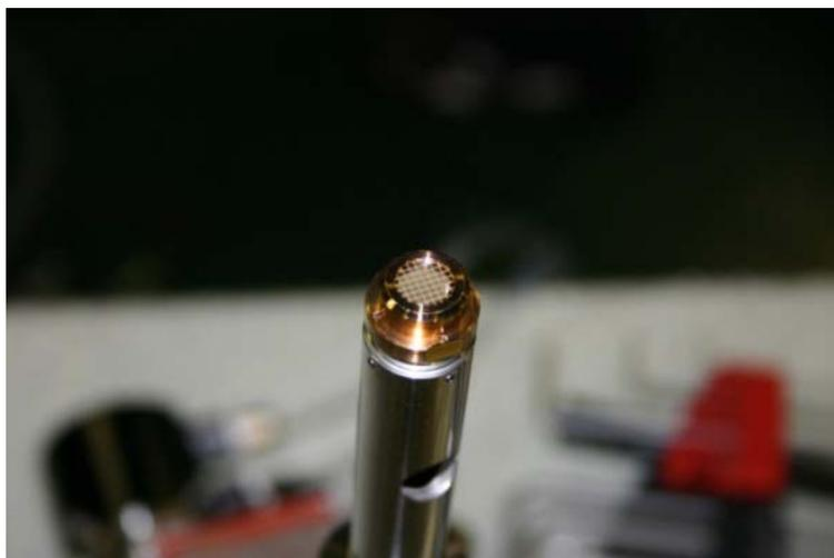
**Fig. 2 The photograph of the tip of a poly-capillary**
