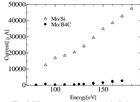
Fig. 2 PD current at 3rd harmonic light without filter.
