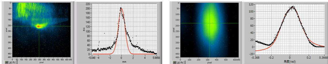
Fig.4 Observation of Optical Transition Radiation (OTR). Beam spot image and data fitting in vertical direction (left). Beam divergence and data fitting in vertical direction (right).
