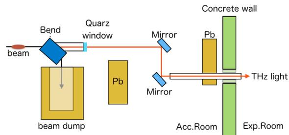
Fig.5 THz beam-line.
