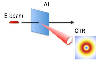
Fig.3 Optical Transition Radiation (OTR).
