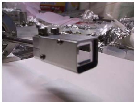
Fig. 1 Photodiode detector. The electrode leads were covered with an Al plate.
