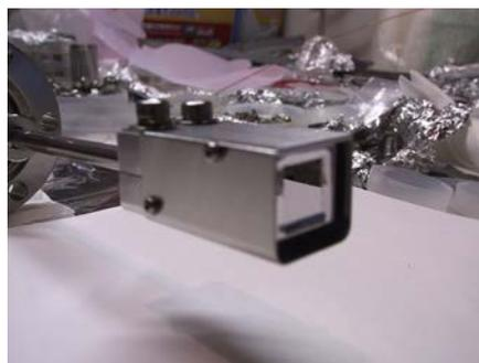
**Fig. 1** Photodiode detector. The electrode leads were covered with an Al plate.
