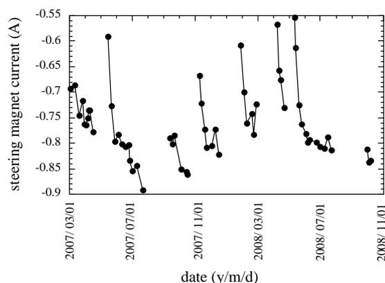
Figure 2: Example of the change of a steering magnet current after the COD correction. The average current of six horizontal steering magnets at dispersion sections is plotted. The values in the same operation cycles were connected with lines. A current shift of 0.1 A corresponds to an rf frequency shift of 2.1 kHz/500 MHz, or a maximum horizontal displacement of 3.4 mm.
