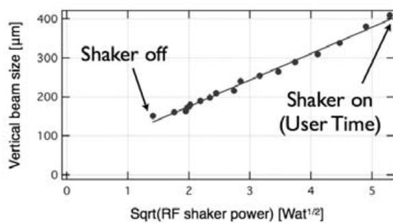
Fig.2. Vertical beam size vs. RF shaker power
