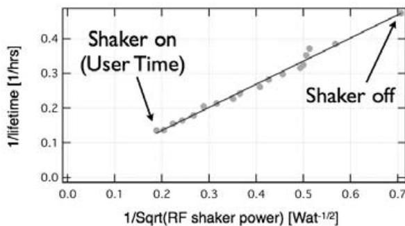
Fig.1. Lifetime vs. RF shaker power
