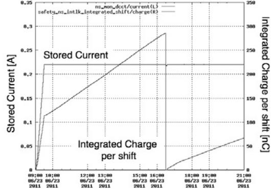
Fig. 4. Beam accumulation and top-up operation in a day
