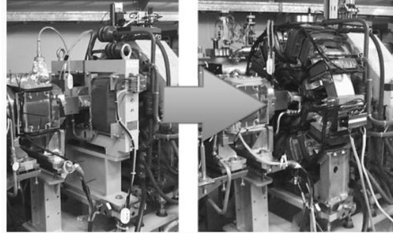
Figure 3: Four vertical steering magnets in the dispersion section were replaced by the multi-element corrector magnets.
