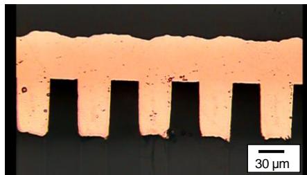
Fig. 3: SEM image of coil lines after copper electroforming
