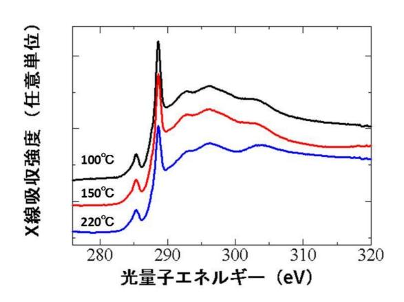
C-K edge XANES spectra of MMA- MAA co-polymer films with TGDDM at various temperature
