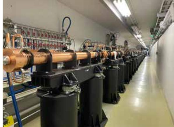
Fig.3. C-band accelerating structure of the 1.0 GeV linac.
