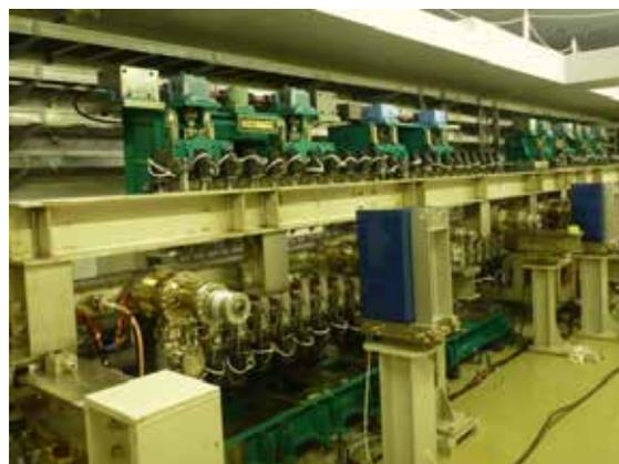
Fig. 5. Insertion device for generating mono-cycle FEL light pulse. Modulator and radiator with high K parameter and a magnetic chicane between them.
