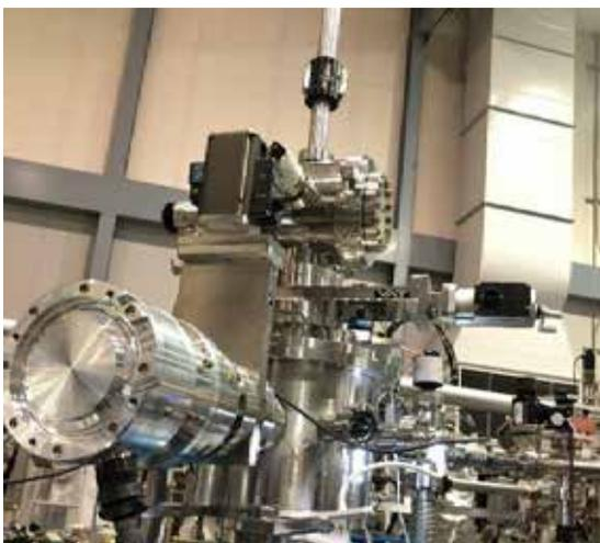
Figure 11. the hydrogen embrittlement evaluation tool of EUV masks and resist.
