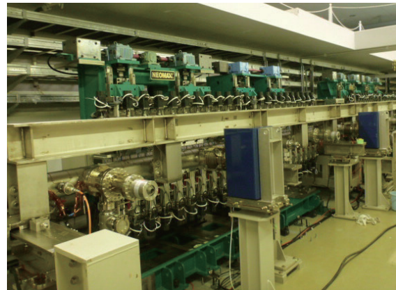
Fig. 3. The new insertion device for generating mono-cycle FEL light pulse. Modulator and radiator with high K parameter and a magnetic chicane between them.
