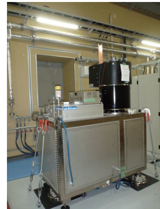
Fig. 9. C-band klystron installed at the klystron gallery for the new injector.
