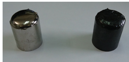
Fig1. Bulk amorphous alloy (left) and crystalized one by annealing of the amorphous alloy (right).
